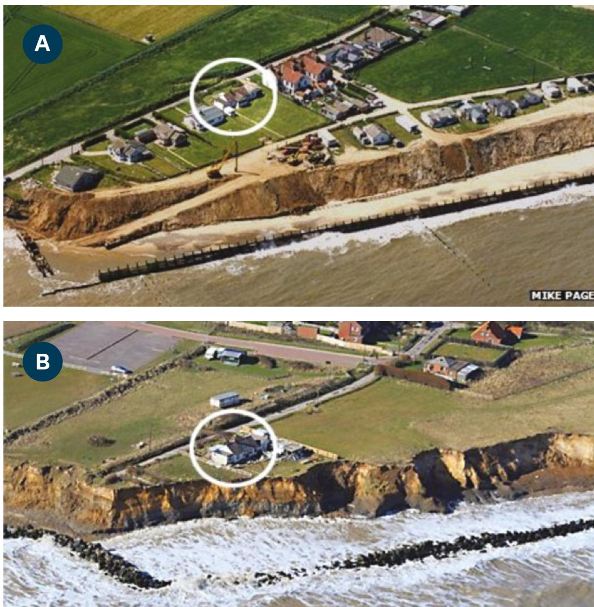
*Figure 2: Photos taken in 1998 (a) and 2013 (b) at Happisburgh. Cliff erosion has left the property just metres from a sheer drop to the beach. Other houses have been demolished. Photos: © Mike Page 2016 ([www.mike-page.co.uk](http://www.mike-page.co.uk)).*
