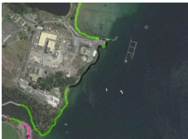
Figure 5: Smartline map results for the Electrona Wharf show it is located in an area of low erodibility. Source: © CoastAdapt 2016b.
