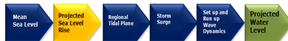
Figure 13: Components of water levels for the open coast. Source: Developed by the author.
