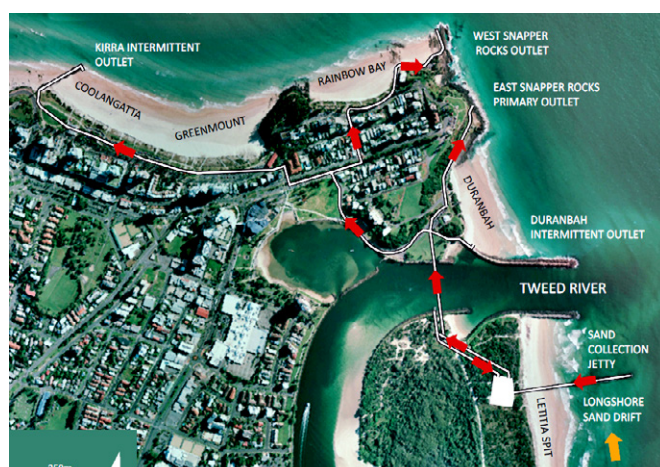
Figure 21: Tweed entrance bypassing scheme. Source: © The State of New South Wales (Tweed River Entrance Sand Bypassing Project) 2016.
