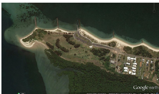
Figure 20: Part of the groyne field at Silver Beach, Kurnell, NSW. Source: ©Google Earth.
